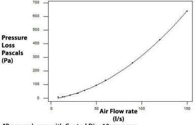
\*Pressure losses with Control Disc 10mm open
