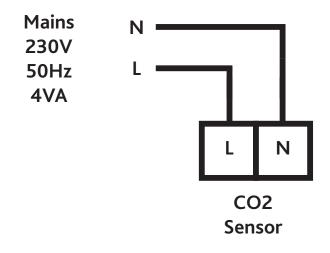
The CO2 sensor requires a 230V power supply. Remove the front panel as per the humidity sensor and release the terminal cover via a fixing lug on the rear of the sensor. Refer to the wiring diagram provided and connect the supply to the terminal box. Finally the sensor may be mounted to the wall (screws are not provided).
