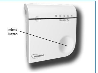
The front panel of the sensor must first be released by pressing in the plastic fixing lug located on the bottom edge of the sensor. The panel may now be removed and the sensor mounted on the wall in a suitable location (screws not provided). 2x AA batteries are provided.
