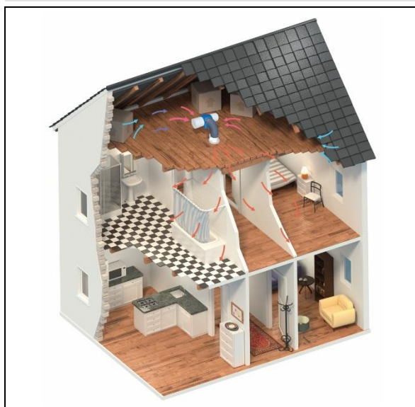
Figure 1 Loft-mounted ventilation unit
