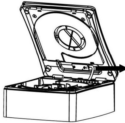
Fig. 6. PIR sensor cable - ( TM only )
