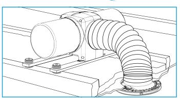
Place anti-vibration mounts above and below each batten fixing point and, using the 4 large screws and special washers, fix the unit to the joists.
