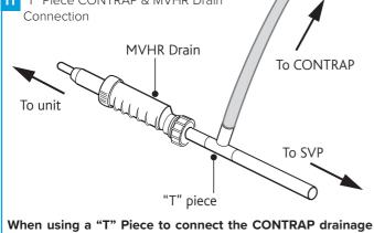
when using a "1" Piece to connect the CONTRAP drainage and the MVHR drain pipework the MVHR drain must always be fitted before the "T" Piece to prevent condensate from feeding back into the MVHR system.
