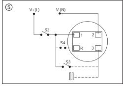
RESET: To reset the counters or hour meters to zero a voltage, with the range of the individual unit, must be applied to terminal R. A non-latching push button is recommended for this.
