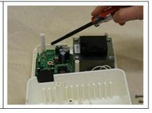
If both these checks are OK, the problem lies within either the wiring or connection from the fused spur to the transformer.
