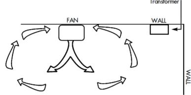
**m)** The Transformer / Humidity sensor unit may be mounted on the wall or ceiling.
