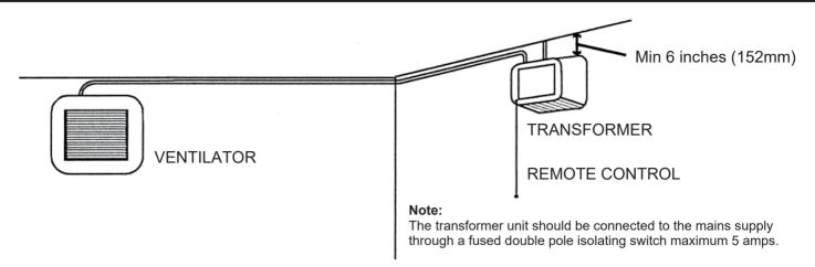
The Heat Recovery Ventilator is a "SELV" (Safety Extra Low Voltage) ventilator that operates at 12 volts AC. Under no circumstances must this be connected directly to the mains supply. Damage so caused is not covered by the warranty. The isolating transformer / humidity sensor supplied must provide the low voltage used by the ventilator. A typical layout of installation is shown above.
