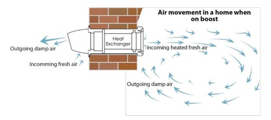
The ventilator runs continuously at trickle speed providing background ventilation. The two airflows pass through alternate layers of a highly efficient aluminium heat exchanger. The incoming air collects the transferred warmth, without mixing the airstreams. Should humidity rise above a preset level, the machine will switch to boost mode rapidly exchanging the air to bring the humidity down. Having achieved this the machine will switch back to normal trickle speed.
