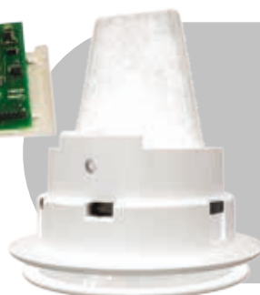
Q-AIRE-EV125FH Extract Valve with filter and fitted integral humidistat
