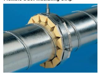
A highly versatile insulation system manufactured from high density phenolic foam which provides a new and improved solution to the requirement for structural insulation where ducts and pipes are supported. Fire resistant - Class 'O' rating.
