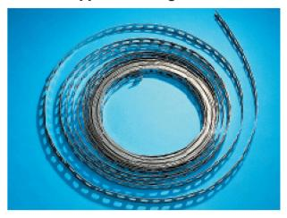
Manufactured from corrosion resistant galvanised mild steel strip 0.9mm thick, and supplied in 30 metre coils. The elongated holes are punched at 30mm pitch to simplify alignment and fixing. Complies with the requirements of DW144.
