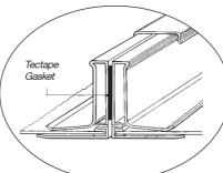
**Note:** 15mm x 4mm x 8 metre size recommended for Ductmate flange system.
