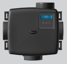
Sentinel Multivent continuous mechanical extract ventilation, MEV is designed for the simultaneous ventilation of separate areas in the home or as a multipoint extraction system for a wide range of commercial applications. The units can be installed at any angle. Where the ambient air has a high humidity content condensate drains are provided.
