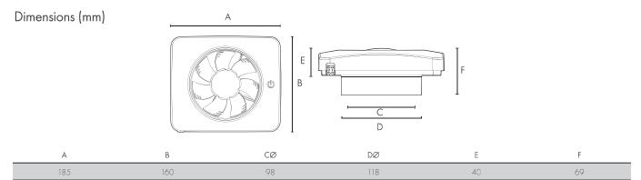
Product is supplied with a removable spigot 30mm deep for  $100 \text{mm} \varnothing$  and  $125 \text{mm} \varnothing$  applications. Weight 1.75 kg
